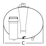
For models O 2000 and larger, vessels are equipped with spray ball cleaning (with detachable cleaning pipe).
