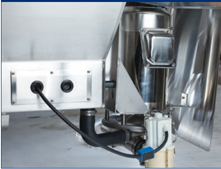
24 V NORMALLY OPEN DRAIN VALVE
